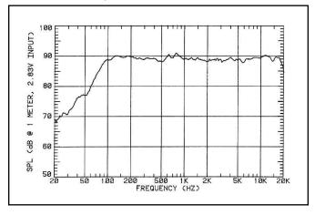
Response curve is an average of five measurements: on-axis, 15 degrees left and right off-axis, 15 degrees up and down off-axis
